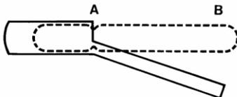
Side view of ampoule opening device containing an ampoule positioned ready to open. 'A' is the score mark and 'B' the point of applied pressure.
